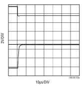
Figure 3a. As soon as the control signal (top trace) changes the MUX channel, the LT6020 output (bottom trace) transitions from the voltage on the previous channel to the next channel. The middle trace shows the input to the multiplexer, with almost no voltage glitch.
