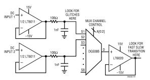
Figure 1. Multiplexed system. LT6011 buffers at inputs have high input impedance. The LT6020 after the MUX can slew fast when MUX changes channel. LT6020 special input circuitry avoids voltage glitches at MUX inputs.
